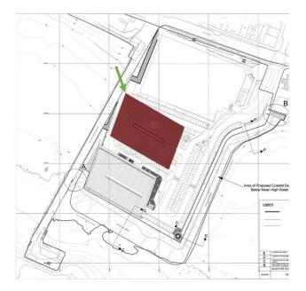
This building would be protected from wave overtopping, but the overall site layout would be inconsistent and inefficient.
